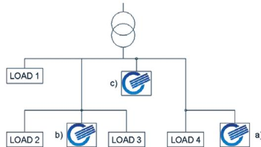
Figure 1: Installation of enclosed capacitor banks
