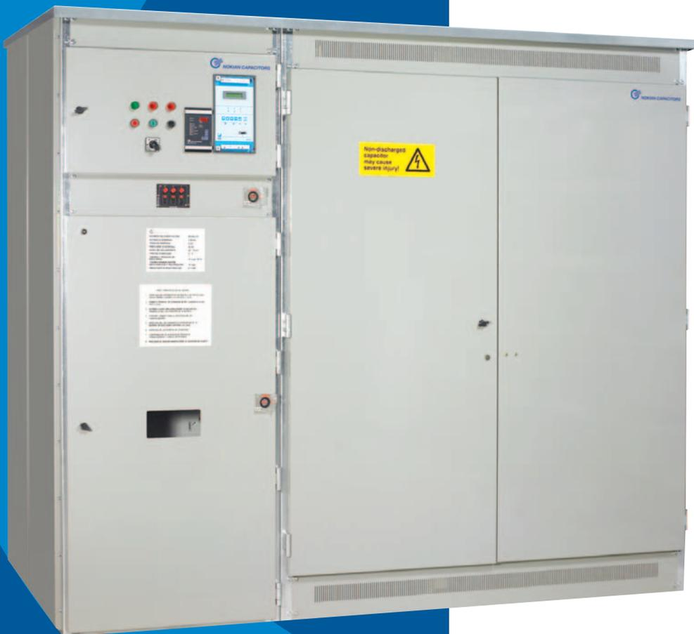
Enclosed capacitor banks designed by Nokian Capacitors Ltd. are used for power factor correction, voltage support, harmonic suppression and to maximize network capacity in industrial applications and distribution systems. They supply individual, group or central reactive power compensation of fluctuating loads in three-phase networks from 3 kV up to 36 kV.
