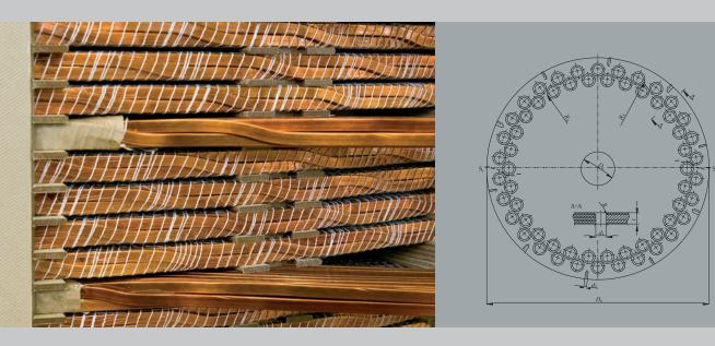
**Continuous disc windings** are made of several numbers of equal coils or sections connected in series. These windings are of advantage when used for transformers rated above 2500 kVA and rated voltages upto 145 kV. channels in the wind ing. Moreover, it does not set high limits for the trans position factor, the crossing wires between stacks can be additionally protected and the winding does not need the polyester netting tape.
