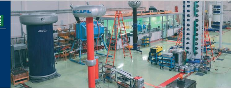
Upon the completion the transformer is subjected to routine test and measurement required by the standards, while each new transformer type also demands type testing. With highly experienced and professionally trained group of employees we can perform routine, type and special tests, required by international standards. The main equipment of the high-voltage laboratory is:
