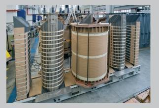
Clamping of windings and of the magnetic core is also important for the transport, where compactness of design assures safe transport without damages, internal movements or slipping transformer within the active part.
